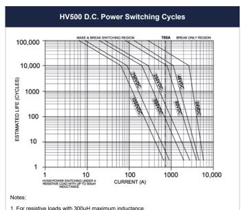
End of life is reached when insulation resistance is < 50MΩ @ 500V.</li>
